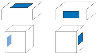
Ventus 920 can apply a label on top, to the side, in front or to the back of a product.
